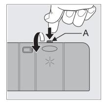
Add the rinse aid in the container. The maximum level for filling is indicated by "max".
